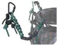
The Aero lineman's belt comes to you already assembled, attached to the Aero saddle, and chained to keep the rope in order when it is not in use. (To release the chain, remove the carabiner from the green loop and pull the rope—the chain will slip out.) It consists of 1) 10 feet of climbing rope, 2) fabric rope sleeve, 3) black 9mm cord, and 4) double-locking carabiner.
