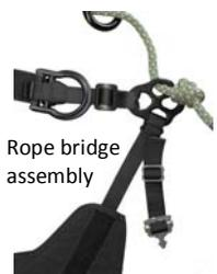
For the rope bridge, rigging plates must be installed on the saddle as described above. The rope (with the ring) is attached to the rigging plate using stopper knots, described below.
