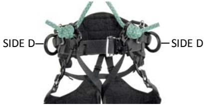
Using a lanyard or flipline, you can also tie in safely to BOTH side Ds. Do not rely on one side D alone. The life-safety structure of the saddle requires that the side Ds be used together. While tied in to the bridge, you can attach a secondary line to just one side D for positioning only. It is also safe to tie in directly to BOTH rigging plates or BOTH shackles in the same way.
