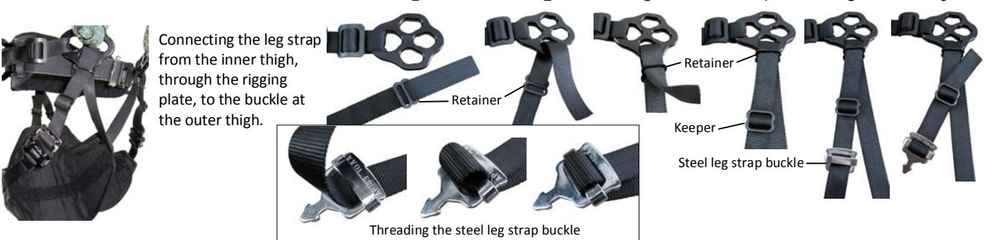
(1) Thread the inner thigh leg strap through one side of the retainer as shown. (2) Pass the strap through the lower hole in the rigging plate, from beneath. (3) Thread the strap through the other side of the retainer. (4) Slide the retainer up close to the rigging plate, then thread the keeper onto the strap. (5) Thread the strap into the steel leg strap buckle as shown, allowing at least 3 inches of tail past the buckle. (6) Thread the tail through the keeper.
