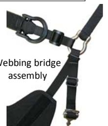
For the webbing bridge, the belt and leg straps are connected in the same way, using shackles instead of rigging plates. The webbing bridge is constructed with an eye at each end for secure attachment to the pins of the shackles. Put the ring on the bridge before closing the shackles.
