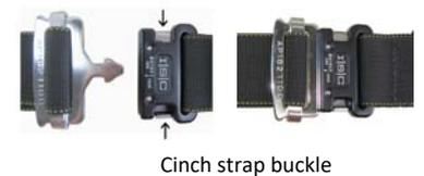
*The cinch strap on the belt holds the saddle in position on your body as you move your weight on and off the saddle during a climb. To open the buckle, squeeze the sides. To close, push the two parts together until they click. Pull the strap snug.*
