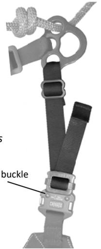
Each leg loop passes through a rigging plate hole. There is a retainer strap attached to the leg loop with two 3-bar slides. This retainer strap restricts the leg loop from sliding too far through the rigging plate, which could cause the leg pads to rotate out of position under your thighs. After you have set the length of the leg loops, adjust the retainer strap to a position on the leg loop that keeps the leg pads centered under your thighs.
